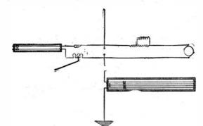
Fig. 1.-Diagram of Arc Method of Transmission.
