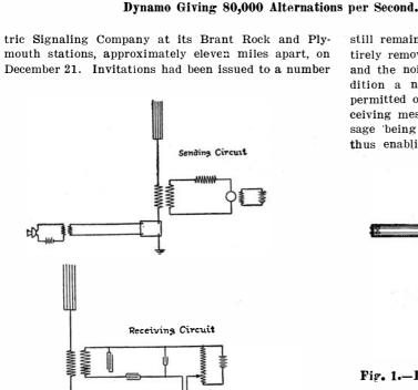
Fig. 3.-Connections for Relay System.
