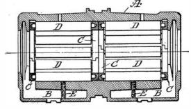
SECTION SHOWING CONSTRUCTION OF ROLLER BEARING.
