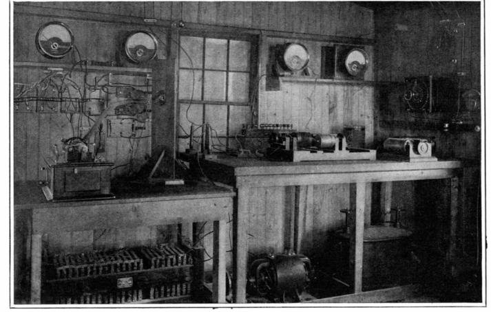
Testing Sensitiveness of Transmitters by Means of Phonograph Records. RECENT PROGRESS IN WIRELESS TELEPHONY.
