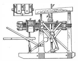
SECTION SHOWING DETAILS OF THE BLOCK MACHINE.
